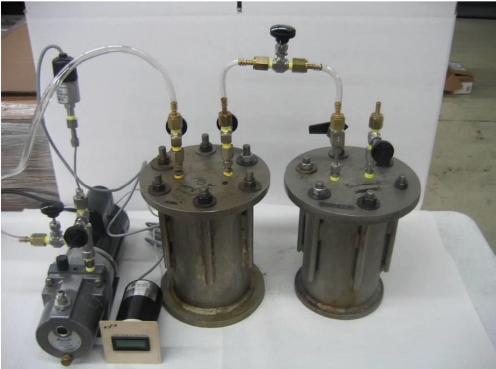
Figure 2 Liquid filling of the sample tank from a reservoir tank using a vacuum pump.
