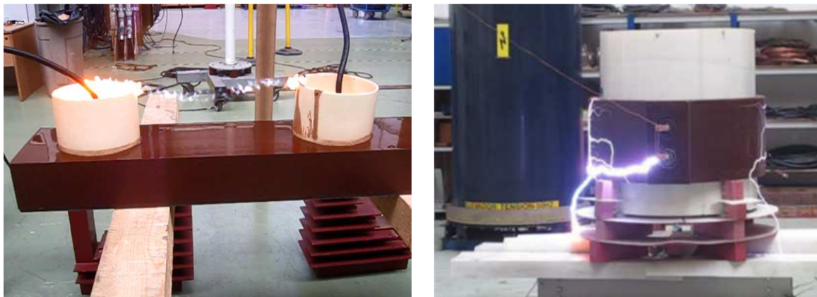
Fig. 3 – Models being tested up to dielectric failure: LI between terminals along the HV winding (left); AC between high voltage and the clamps (right)
