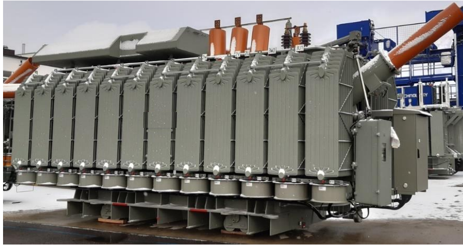
Figure 2: Photograph of the completed 80 MVA unit filled with NYTRO BIO 300X.
