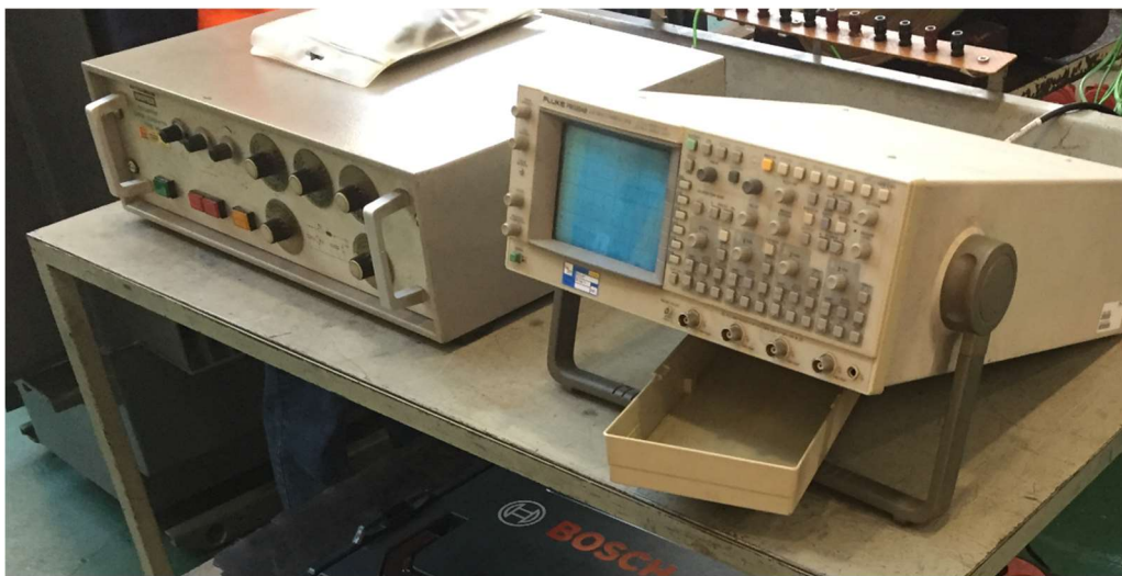
Fig 5. Recurrent surge generator and oscilloscope used on the experiments.
