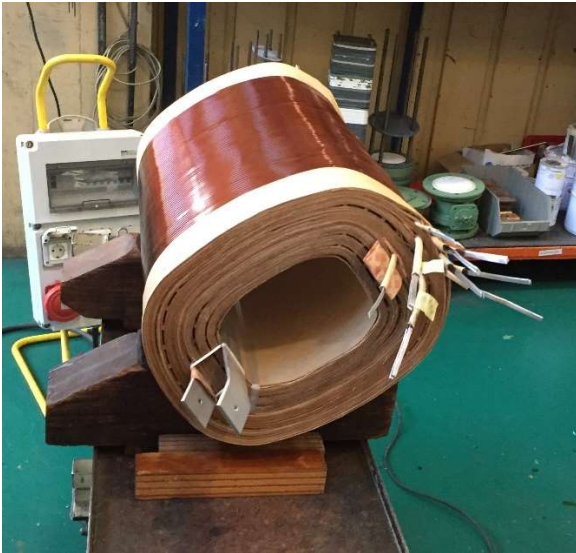
Fig 6a. Single phase tested without core.
