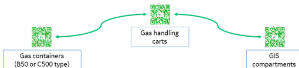
Figure 5-3 - Principle of QR-code based identification
