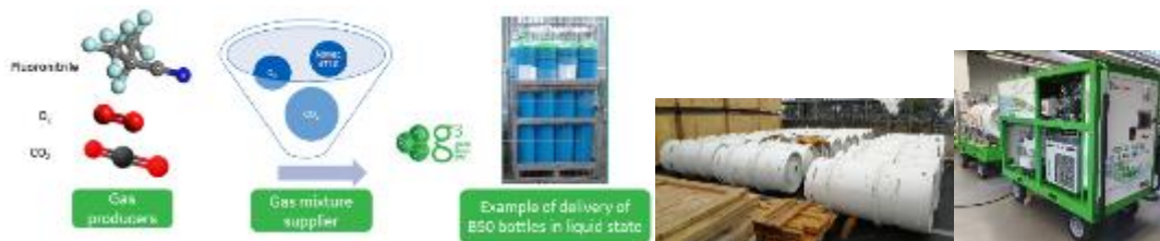
Figure 5-1 – Gas mixture delivery to site in pre-mixed B50 bottles or C500 containers
