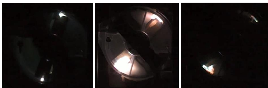
Figure 6: MV Rotary switch high speed frames for contact separation (left), arc elongation (middle) and current zero followed by dielectric recovery (right)
