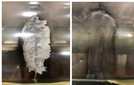
Figure 8: Surface tracking on the arced surface without O 2 (left) and with O 2 (right)
