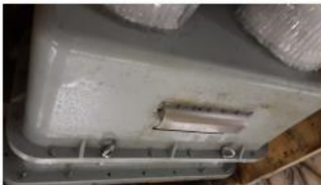
Figure 7 – Rubber Shed Deformation and Corrosion Damage of 600kV CT after Several Seasons of Rain and Winter Freezing Exposure.
