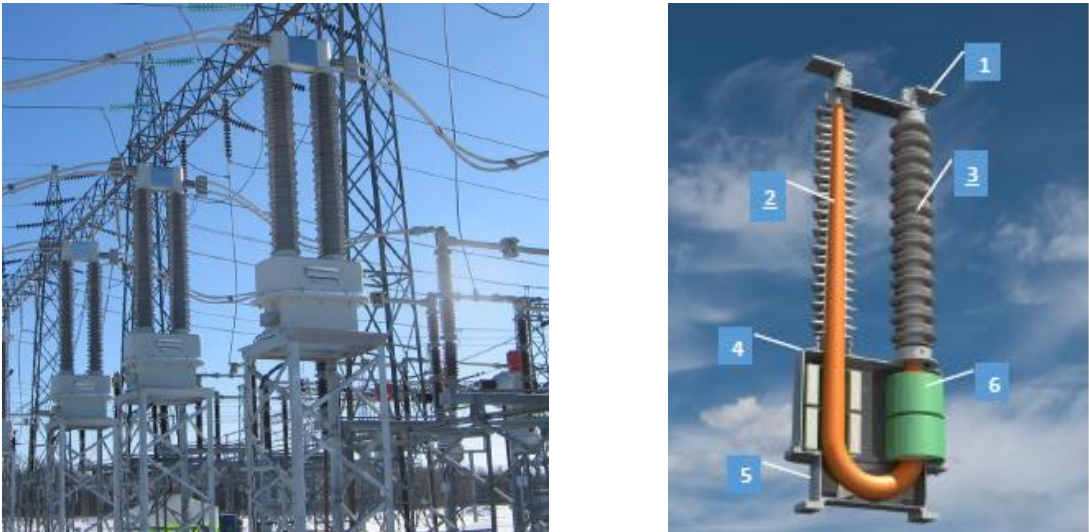
1 – Primary Terminal 2 – Primary Condenser Core 3 – Silicone Rubber Sheds 4- Base Box Upper Casing 5 – Base Box Lower Casing 6 – Secondary Winding
