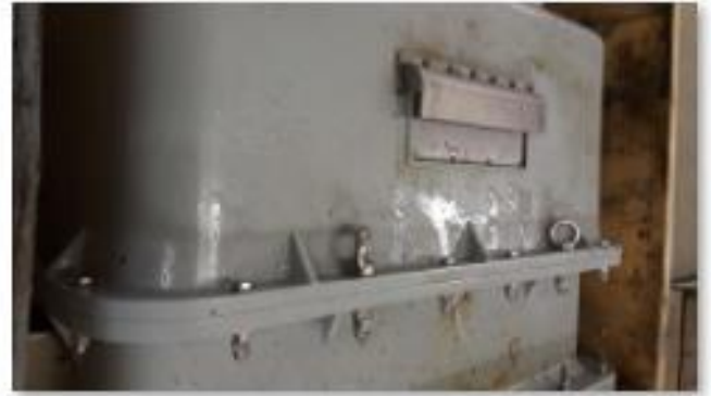
Figure 7 – Rubber Shed Deformation and Corrosion Damage of 600kV CT after Several Seasons of Rain and Winter Freezing Exposure.
