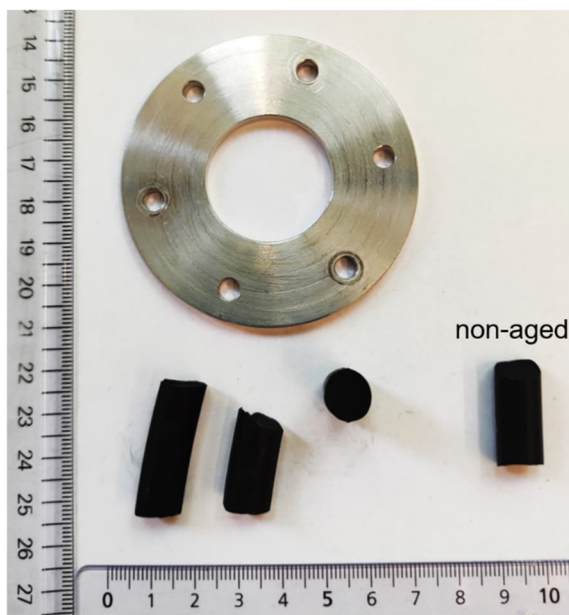
Figure 4 EPDM after 4 weeks at 100°C in C4-FN / O 2 / N 2 mixture
