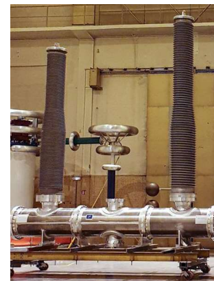
Figure 3 : 420kV GIS circuit-breaker prototype during dielectric test in High Voltage laboratory
