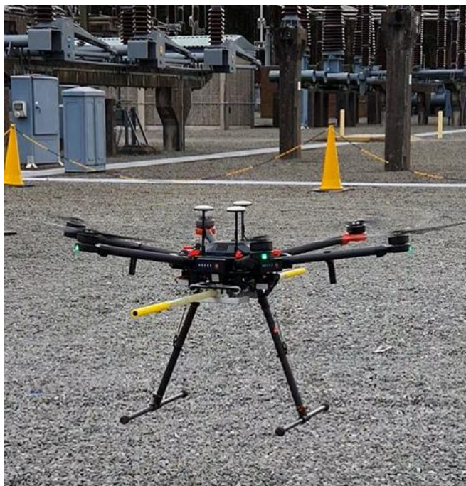
Figure 3 UAV used for the project with PD locator fitted.
