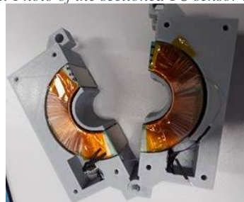
Figure 2: Photo of the sectioned TC sensor developed
