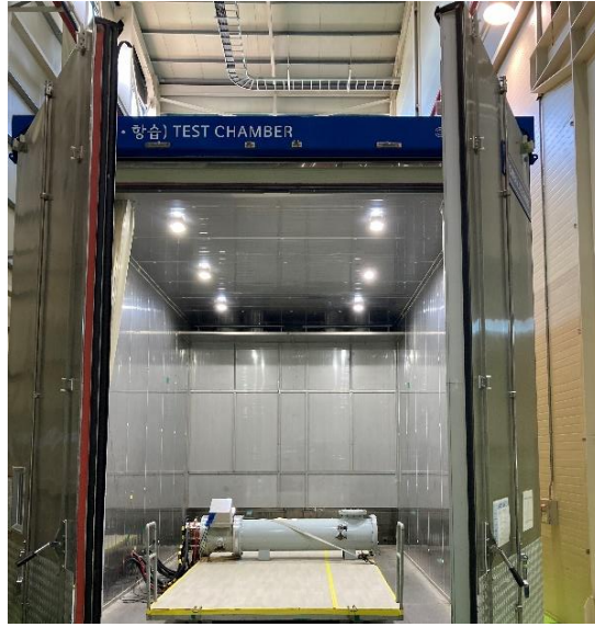
Fig. 9 Test setup of the LPIT in climatic chambers
