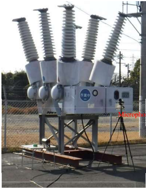
(1) Measuring the operation sound
