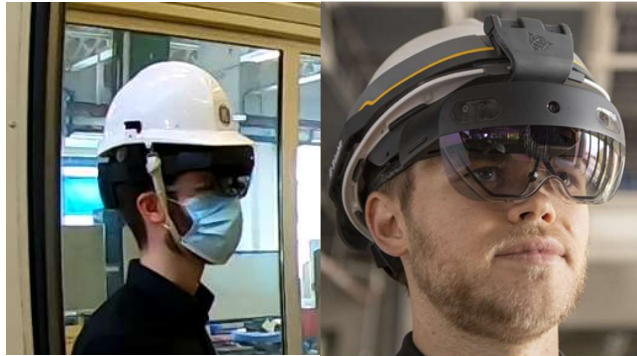
Figure 5: the mixed reality headset can be adjusted to the safety helmet thanks to homologated adapters
