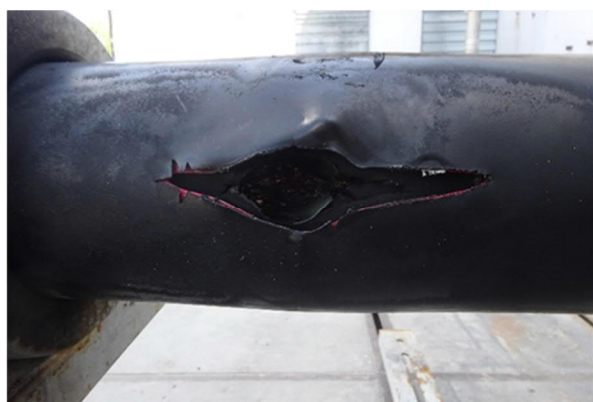
Figure 7: Cable following Test 2
