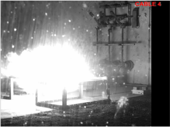
Figure 5: High speed image during fault
