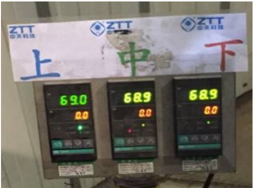
Fig.5 Insulation core temperature monitoring values during degassing process
