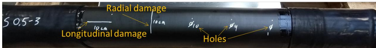
Figure 8: Cable sample with artificial defects machined on the outer PE jacket
