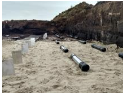
Figure 9: Arrangement of the samples in backfill, before covering and compaction
