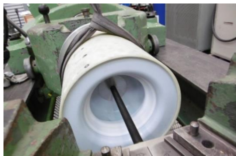
Figure 3: Test to verify the mechanical fixing of the stress cone in the hollow insulator
