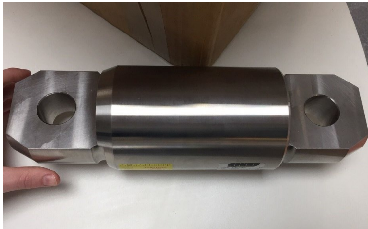
Figure 7 : Photograph of the pulling forces sensor
