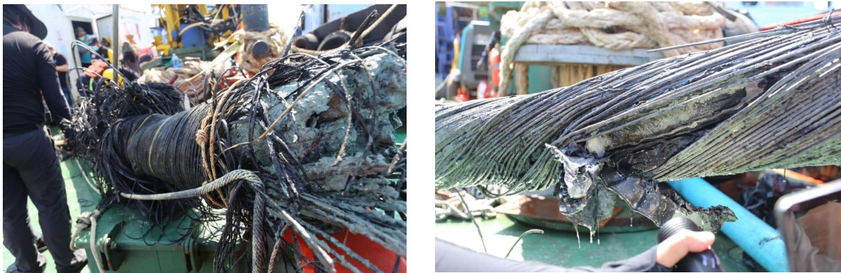
Figure 1: Submarine cable was damaged by Navy ship.
