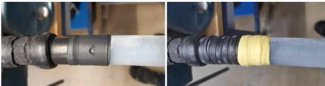
FIGURE 1: THE TEST SAMPLE WITH AN INTERNAL MV FAULT WITH TWO HOLES IN THE INSULATING TAPE INSERTED BENEATH THE SEMICONDUCTING TAPE LAYER.
