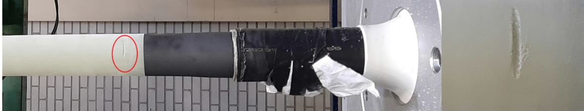
FIGURE 5: TEST SAMPLE WITH AN INTERNAL HV FAULT, WHERE THE INSULATION WAS CUT IN A PART OF THE CABLE BENEATH THE STRESS CONE.
