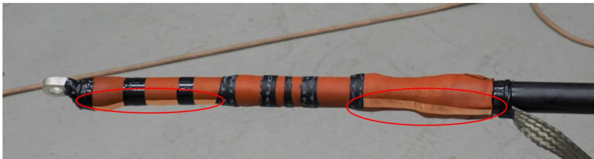
FIGURE 3: TEST SAMPLE WITH AN EXTERNAL MV FAULT, WHERE CLEARANCE BETWEEN LIVE AND GROUNDED PART WAS REDUCED BY INSERTING TWO SECTIONS OF COPPER TAPE (HIGHLIGHTED BY RED CIRCLES) AND ROUNDS OF SEMICONDUCTING TAPE.
