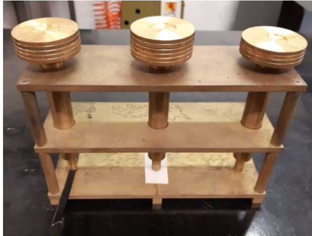
Figure 9 Example of deformation test apparatus with specimens in place
