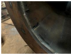
Base plate and stiffener weld
