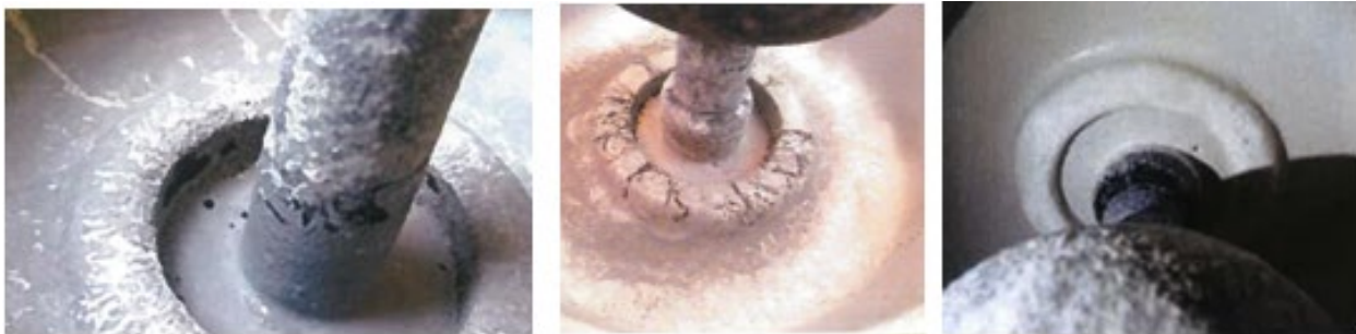
Figure 4: Examples of silicone coated glass insulators using different chemistries of coating after the 2000h test.
