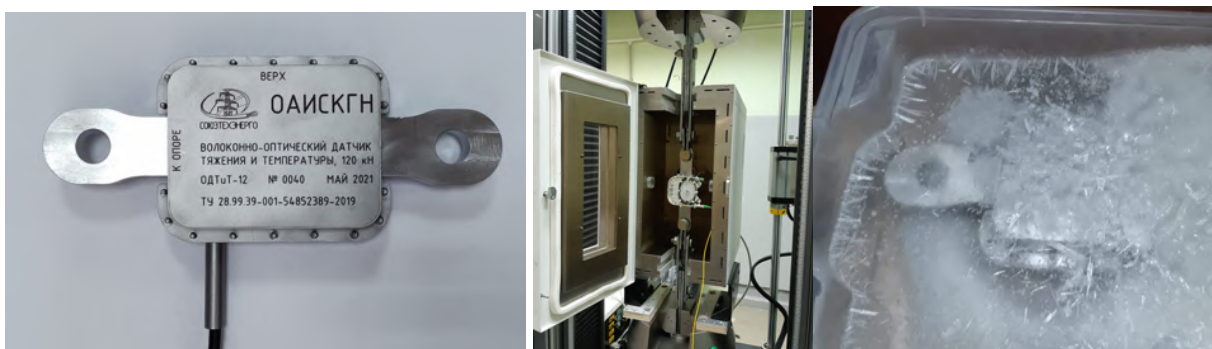
Figure 3 – Left to Right FBG load-cell, testing on a tensile machine with a temperature chamber, freeze-thaw testing
