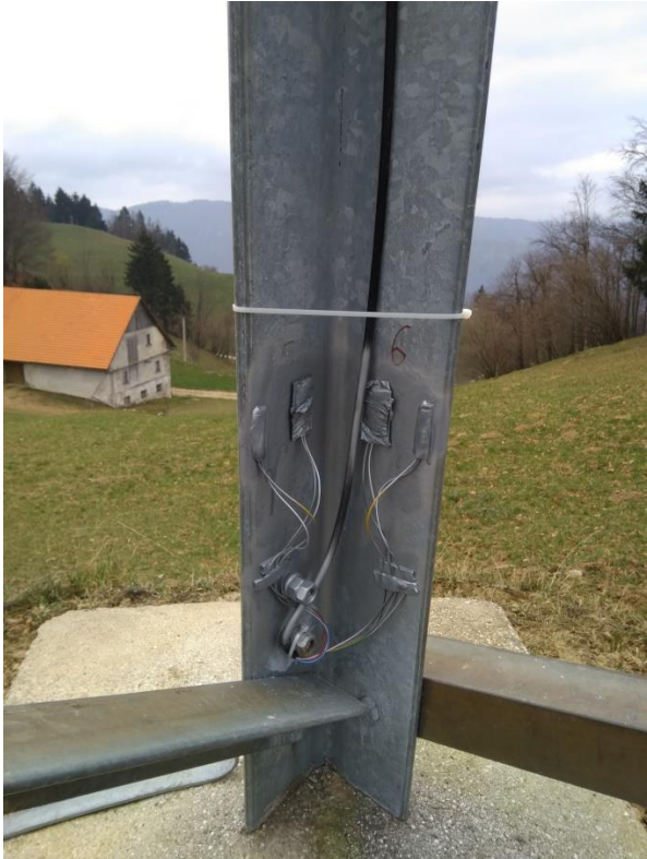
Fig. 2. Adhesive strain gauges at the location of the measured residual stresses on the L profile
