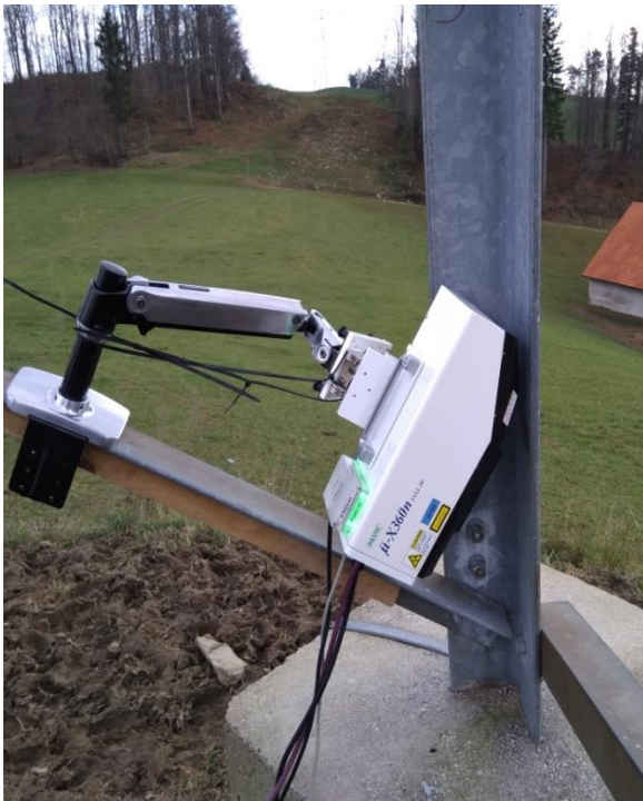
Fig. 1. Measurement of residual stresses on the SW leg at the 6 th measuring point
