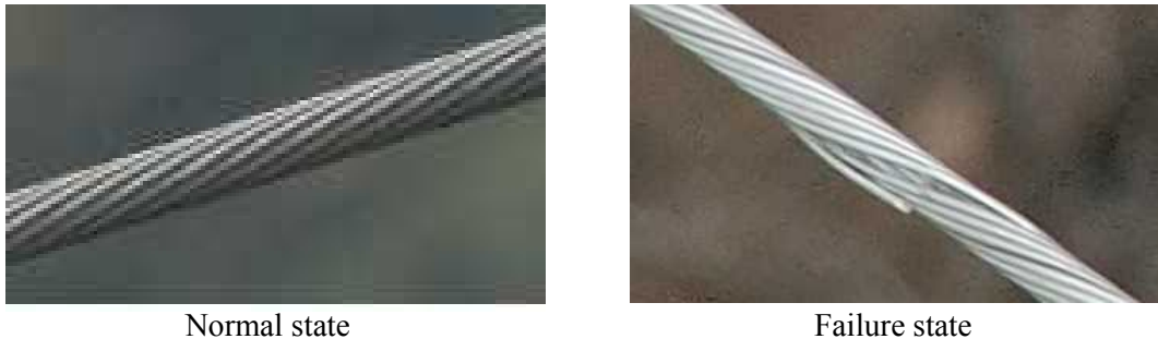
Figure 1. Normal and failure states of conductor
