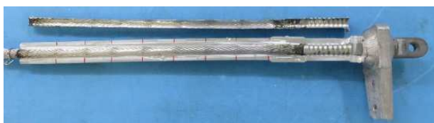
Fig. 8 ACFR inside the aluminum clamp
