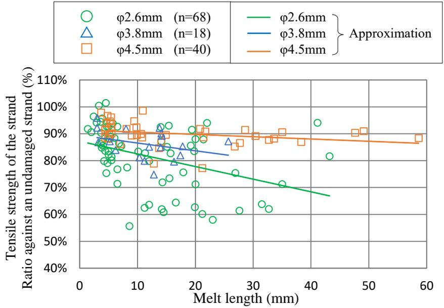
Figure 3 (a) Relationship between melt length and residual tensile strength of melted strands
