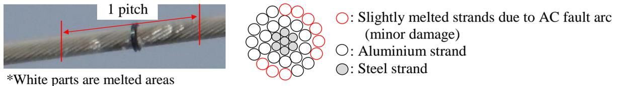
Figure 8 An example of appearance of a damaged conductor for evaluating repair method (ACSR410 mm<sup>2</sup>)
