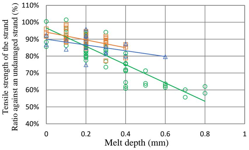
Figure 3 (c) Relationship between melt depth and residual tensile strength of melted strands
