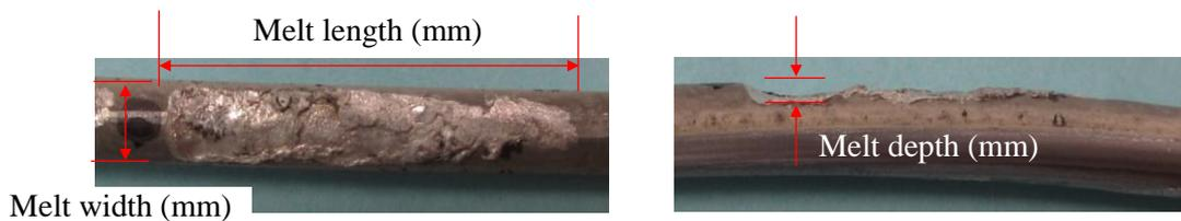
Figure 2 An example of a strand damaged by an AC fault arc
