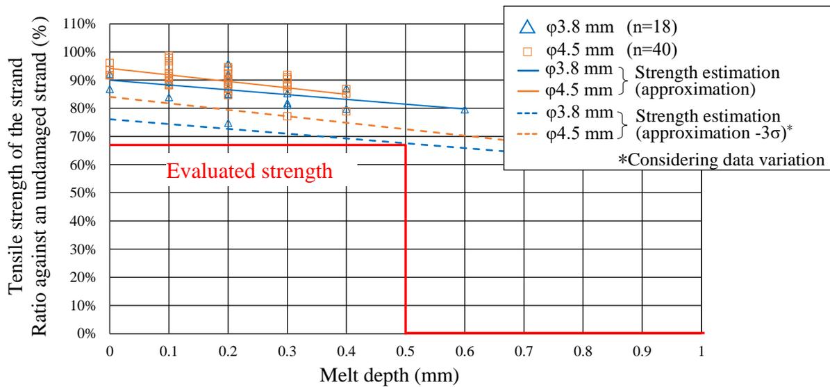
Figure 5 (b) Tensile strength of the melted strand ( $\phi 3.8$  mm,  $\phi 4.5$  mm)
