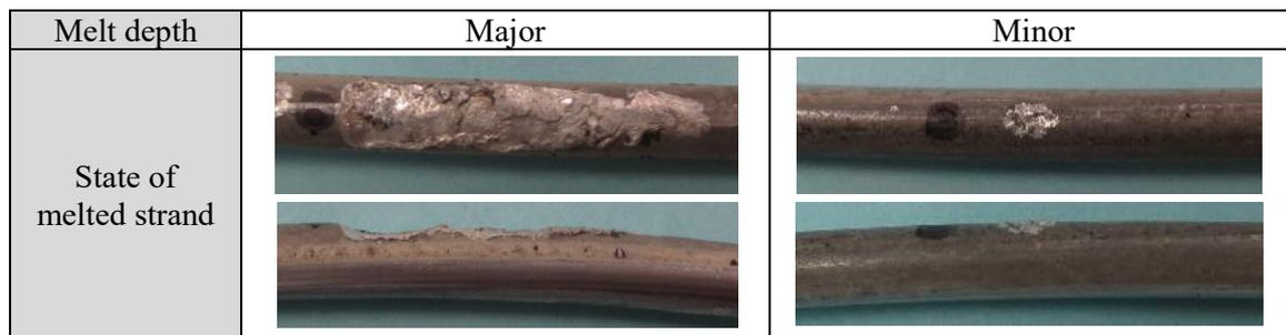
Figure 6 Comparison of appearance of damage level
