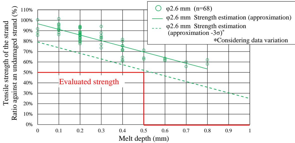
Figure 5 (a) Tensile strength of the melted strand ( $\phi 2.6$  mm)
