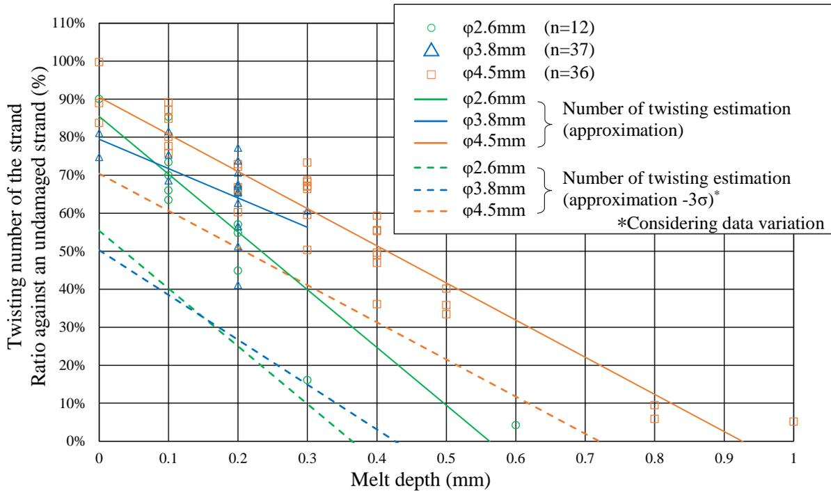
Figure 4 Ductility characteristics of the melted strand
