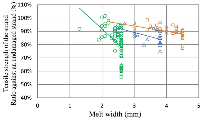
Figure 3 (b) Relationship between melt width and residual tensile strength of melted strands
