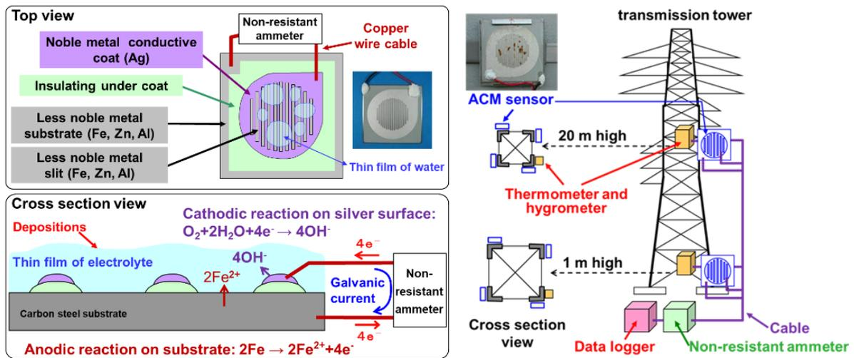
Figure 1. Schematic diagrams of ACM sensor and corrosion monitoring system on transmission tower
