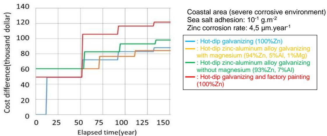
Figure 10. Lifecycle cost differences comparison of transmission towers with different type of galvanizing and factory painting in coastal area (The initial cost of transmission tower with hot-dip galvanizing was subtracted to deliver the cost differences.)
