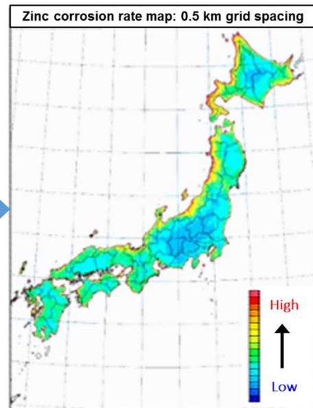
Figure 2. Corrosion rate map of hot-dip galvanizing
