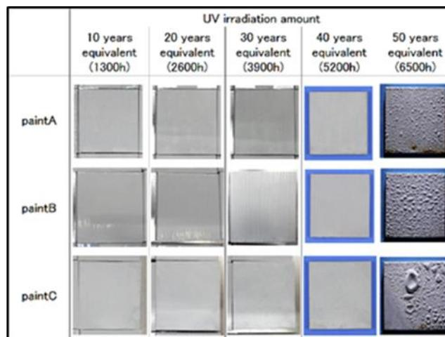
Figure 8. Surface observation result after UV irradiation accelerated degradation tests
