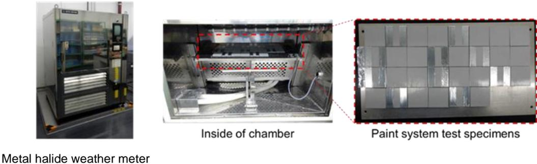
Figure 6. Metal halide weather meter type UV irradiation accelerated degradation test equipment and test specimens
