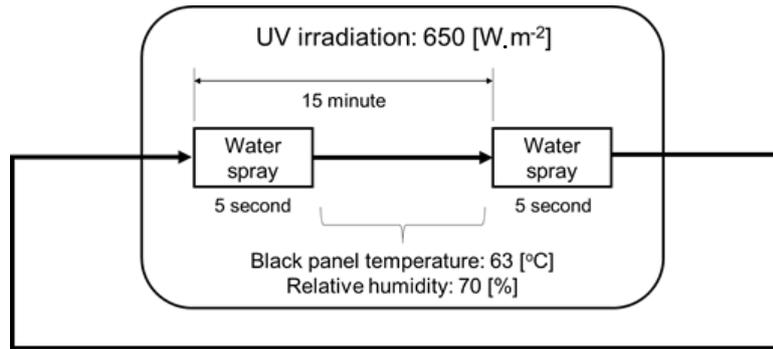
1300 hours of the UV irradiation accelerated degradation test in metal halide weather meter corresponds to 10 years in normal outdoor environments in Japan.
