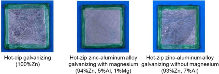
Figure 3. Specimens of hot-dip galvanizing and hot-dip zinc-aluminum alloy galvanizing with and without magnesium for combined cycle accelerated corrosion test
