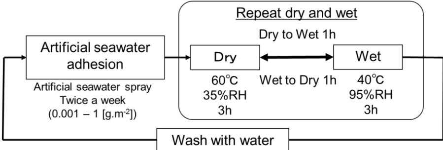
Figure 4. Combined cycle accelerated corrosion test condition according to ISO 16539 [1]
