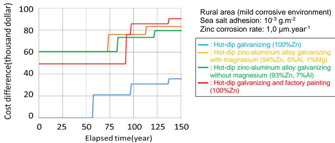
Figure 9. Lifecycle cost differences comparison of transmission towers with different type of galvanizing and factory painting in rural area (The initial cost of transmission tower with hot-dip galvanizing was subtracted to deliver the cost differences.)
