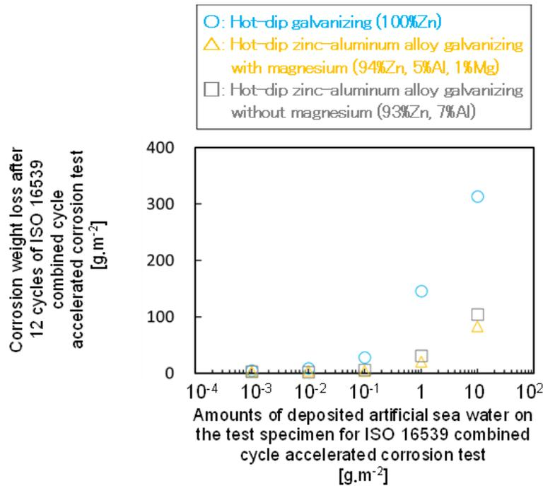
Figure 5. Assessment of corrosion weight loss of hot-dip galvanizing and hot-dip zinc-aluminum alloy galvanizing after 12 cycles of ISO 16539 combined cycle accelerated corrosion test
