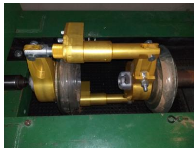
Figure 10 - Arrangement for testing the set of 320 kN equipment and insulators
