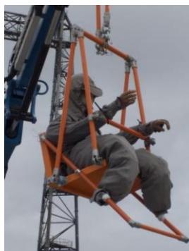
Figure 7 – Simulation of lineman wearing conductive suit and sat on an insulating chair
