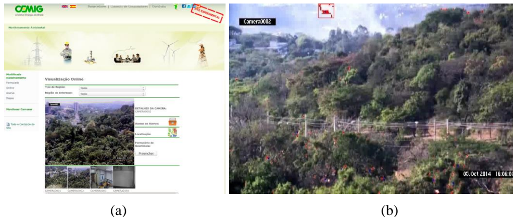
Figure 11 (a) Image of the cameras in the Cemig's intranet, (b) Result of an actual smoke detection that occurred during the pilot test. The upper left red rectangle indicates region in forest near 13.8 kV Distribution Network where the smoke was located.
