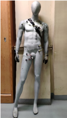
Figure 3 – Conductive skin mannequin with resistor for AC induction testing
