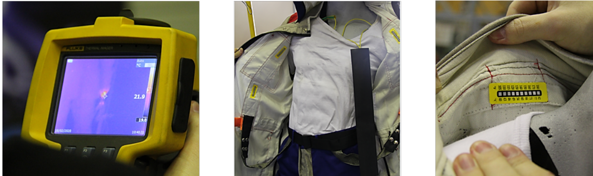
Figure 4 – Thermal indicators: camera (left), 100% cotton clothing (center), irreversible temperature sticker (right)
