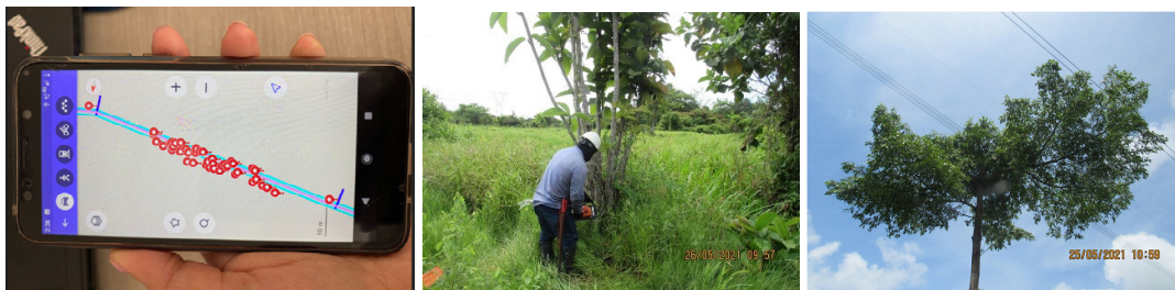
Figure 5 Process to identify and intervened vegetation classify with risk in LiDAR inspection
