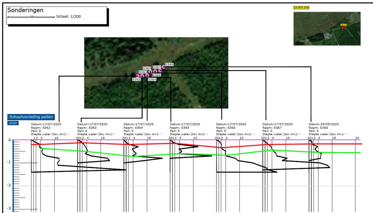
Figure 7 : Geotechnical cross section based on Panda's results -> « type 1 »
