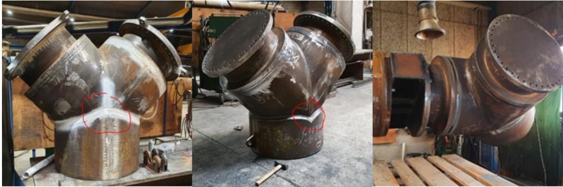
Figure 5 : Left: Center knot type 1. Middle: Center knot type 2, Right: T-knot welded to the shaft
