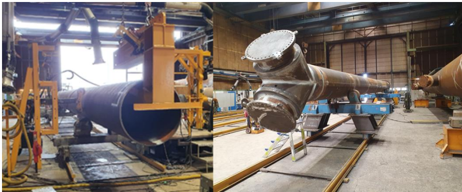
Figure 6 : Left: The shaft is being produced using robots. Right: The shaft/t-knot ready for surface treatment
