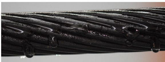
Colored: no continuous wetting, droplets drip off in two lines, not centered
