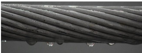
Sand1: almost continuous wetting, recedes quickly, droplets drip off at the lowest point of the conductor
