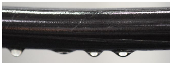
Coated: continuous water film on surface, droplets drip off at the lowest point of the conductor
